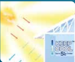
Special pigments reflect infrared radiation back to the atmosphere to keep homes cooler
