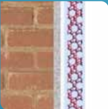
Paint molecules are strongly bonded together, to give superior protection from alkali
